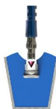
(9) The components are inserted into the repositioning aid, which is located in the impression tray, and fixed in place.
