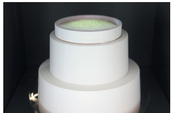
Fig. 5: Optics of the powder after carrying out the cleaning firing for the MoSi2 discolorations: greenish discoloration.
