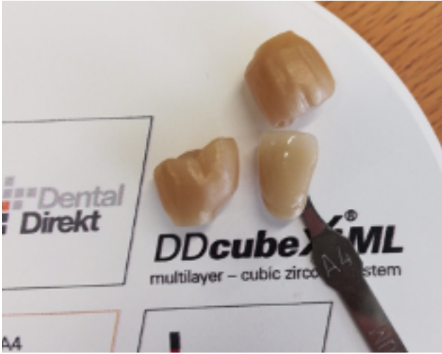
Fig. 14: dark color effect due to insufficient energy input for crowns made of DD cube X2® ML A4
