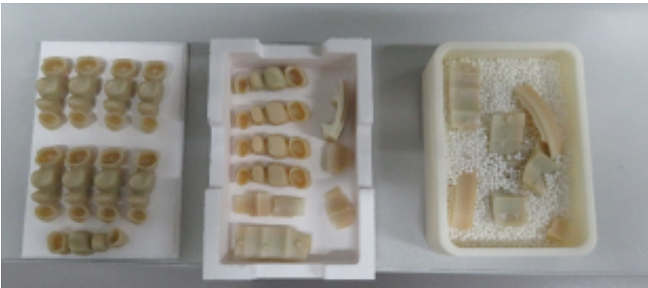
Fig. 9: Again, green discoloration of solid pontics or solid structures
