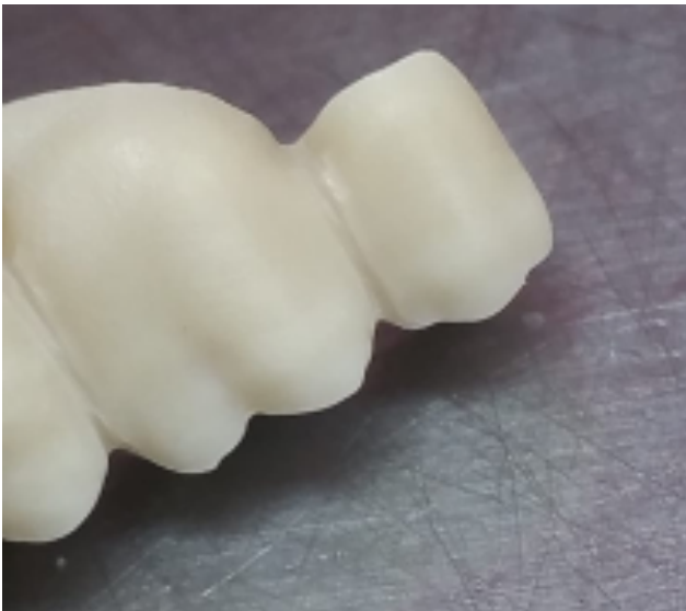
Fig. 15: clearly underbaked construction from DD cube ONE® ML C3: paint layers clearly visible
