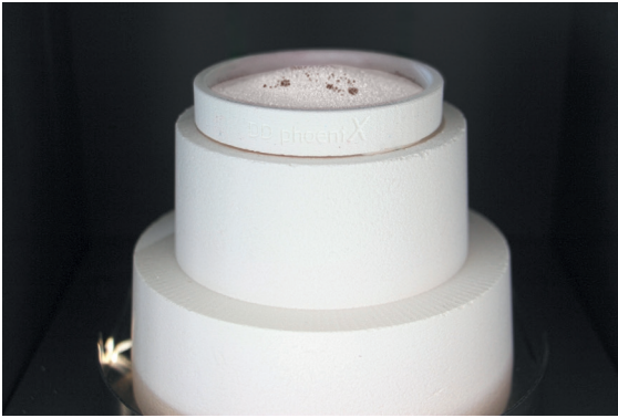
Fig. 4: Optics of the powder after carrying out the cleaning firing in case of deposits: brownish discolored residues
