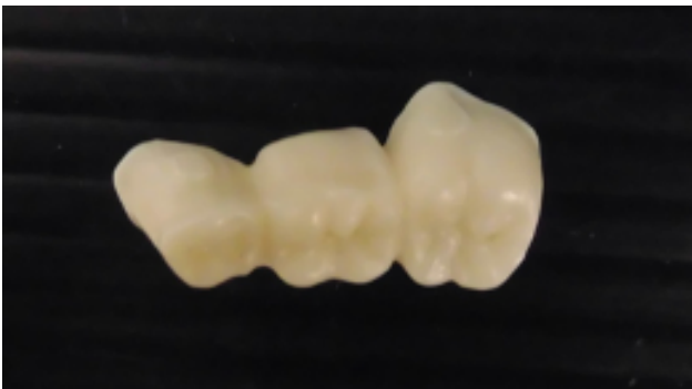
Fig. 16: white crown margins can also be a sign of insufficient energy input: here white crown margin of a DD cube ONE® ML A2
