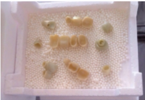
Fig. 8: Green discoloration due to deposited molybdenum(VI) oxide ( \text{MoO}_3 ): stronger discoloration on massive crowns
