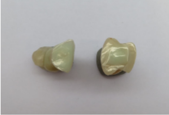
Fig. 6: Green discoloration due to deposited molybdenum (VI) oxide ( \text{MoO}_3 )
