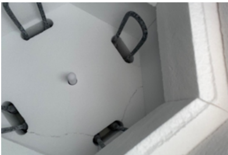
Fig. 1: MoSi 2 heating elements affected by deposits
