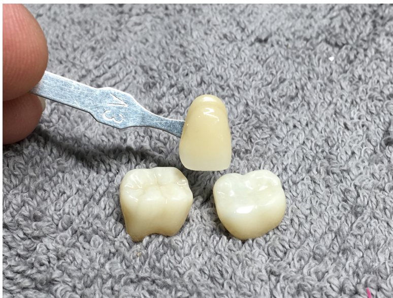
Fig. 17: too light color result due to too high positioning of the crown in the blank
